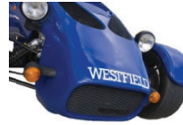
FW Front Single piece nose and bonnet, forward hinged with additional venting.
